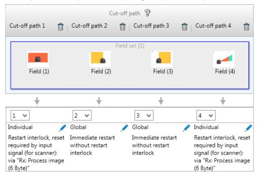
When incorporating the cut-off paths into the logic, the user can select a suitable byte from the assembly. A cut-off path with a protective field or contour detection field is always regarded as safety-related. A cut-off path with a warning field is always regarded as non-safety-related.
