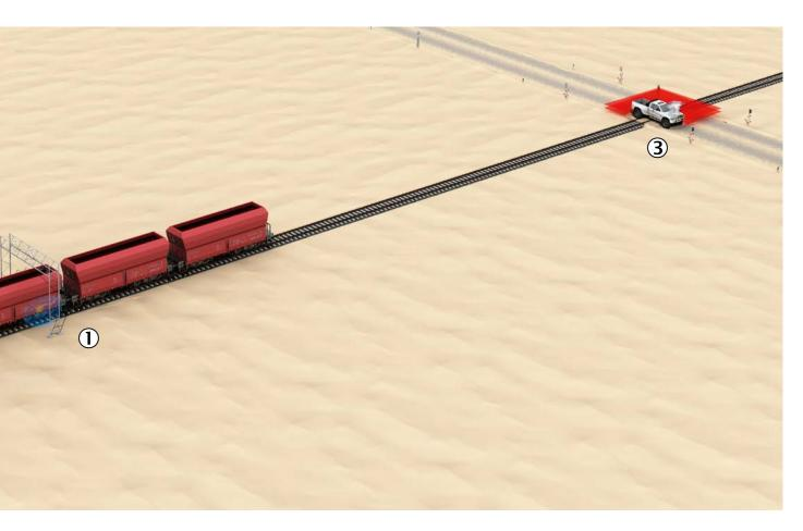
The LMS511 is able to operate in all weather conditions.Combined with the dual channel Flexi Soft safety controller, which continuously monitors the operational state of the laser scanner, a reliable system is provided for level crossing monitoring.
