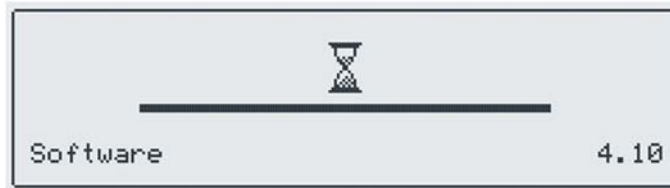
Fig 4: Initial commissioning. The software version is displayed in the lower right corner.
