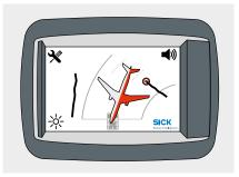
The left side of the aircraft is highlighted in red if the collision object is on the left side of the aircraft.
