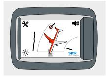
The right side of the aircraft is highlighted in red if the collision object is on the right side of the aircraft.
