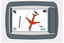
The entire aircraft is highlighted in red if the collision object is behind the aircraft.
