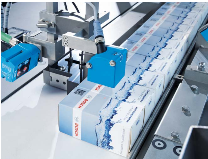
A perfect match: DeltaPac supplies the trigger signal for the Lector62x image-based code reader.
