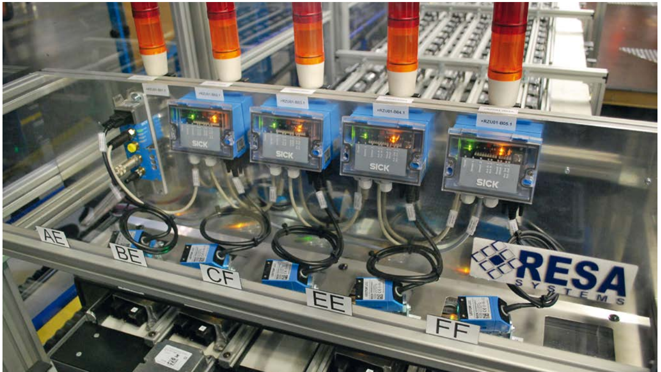
The Lector62x by SICK can be relied upon to read codes on objects that are in motion or stationary, even if the quality of the codes is extremely poor.
