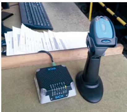
The IDM16x reads the bar codes on the printed assembly orders and the RFU62x transfers the data to a tag.
