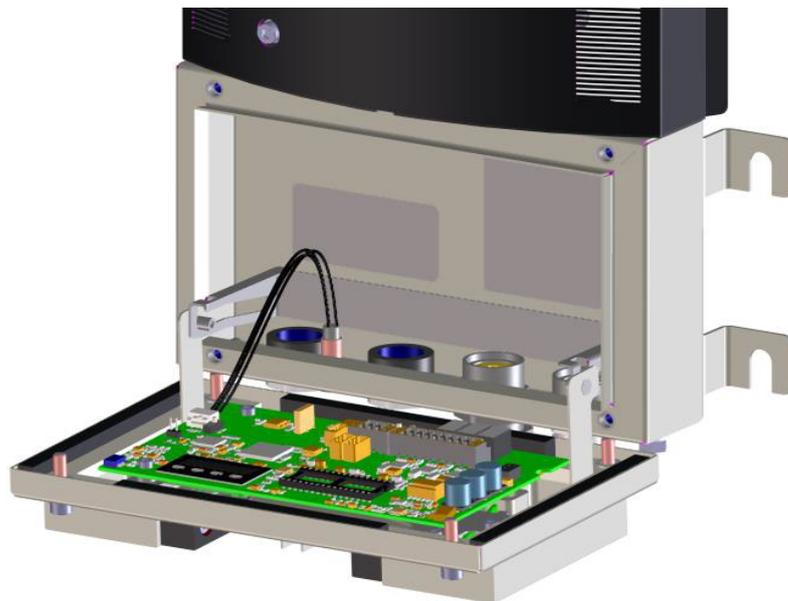
Fig. 24: LED switch position on the mainboard
