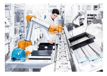
Furthermore, the networking of all components also supports the team play between robots and humans. To ensure this collaboration works equally well for both, DIN ISO/TS 15066 specifies certain safety requirements for collaborative industrial robot systems and the work environment. To meet these requirements, cobots must be equipped with appropriate sensors. These detect people and obstacles in their environment using, for example, infrared, ultrasound or radar technology.
