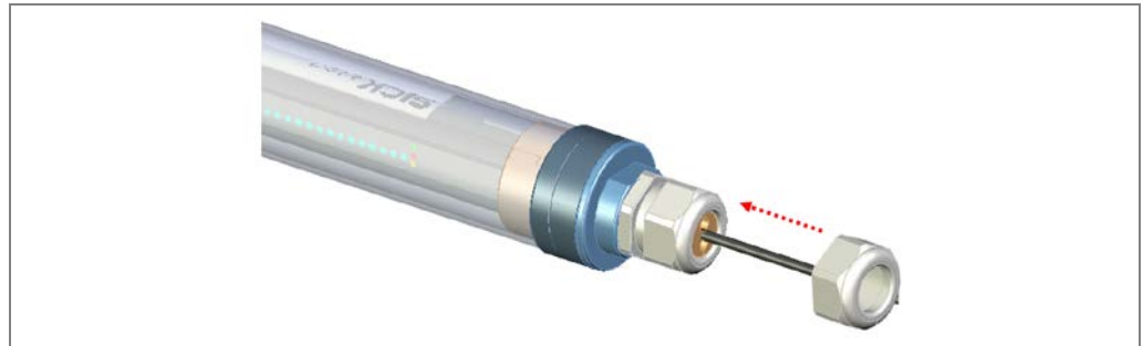
Fig. 47: IPG2: screwing the nut onto the cable gland
