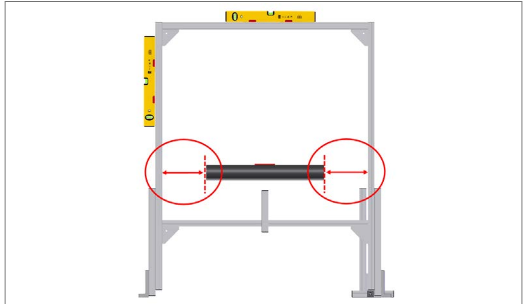
Fig. 29: item mounting frame: aligning the frame
