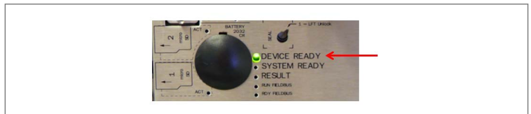
Fig. 118: Checking the operational readiness of the MSC800
