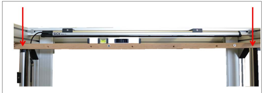
Fig. 57: Checking the alignment of the vertical light grid
