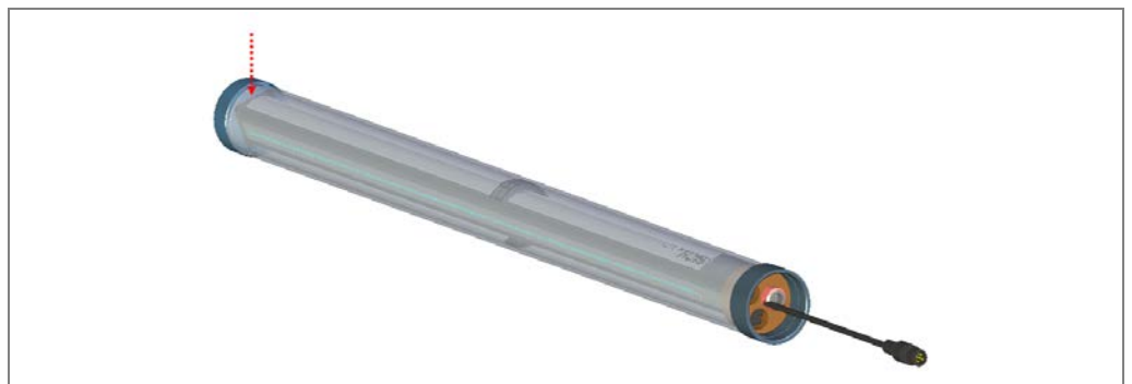
Fig. 43: IPG2: clicking the light grid into place in the upper flange
