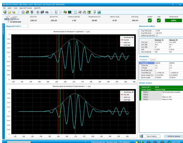
Figure 7 "Path diagnosis" diagram ("Service" user access level)
