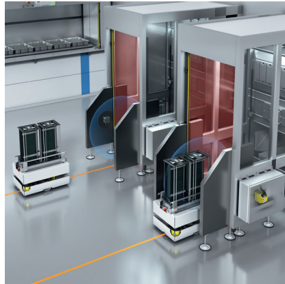
Hazardous area protection during AGV docking with the Safe Entry Exit safety system
