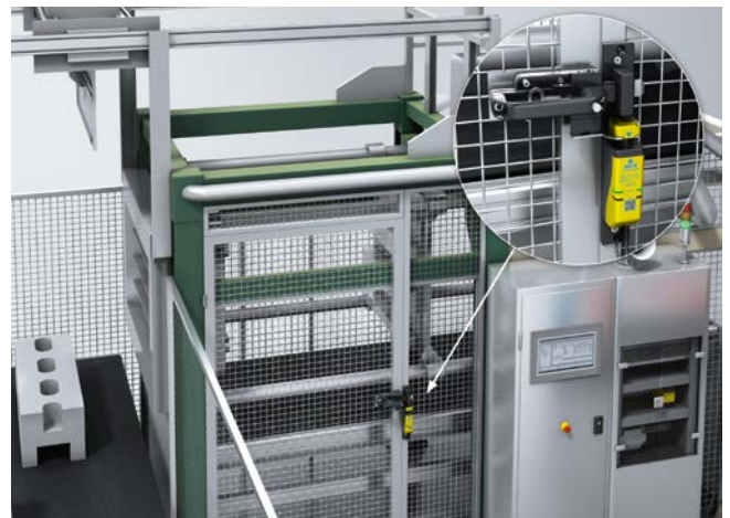
Protection of access doors to a shape molding machine
