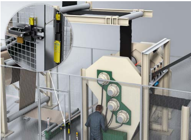
For difficult to monitor calendaring machines, an ANSI-compliant locking mechanism can prevent operators from being inadvertently locked in the hazardous area
