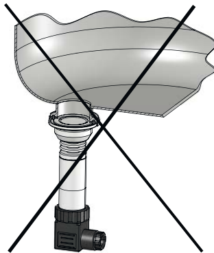
Not self-draining mounting position
