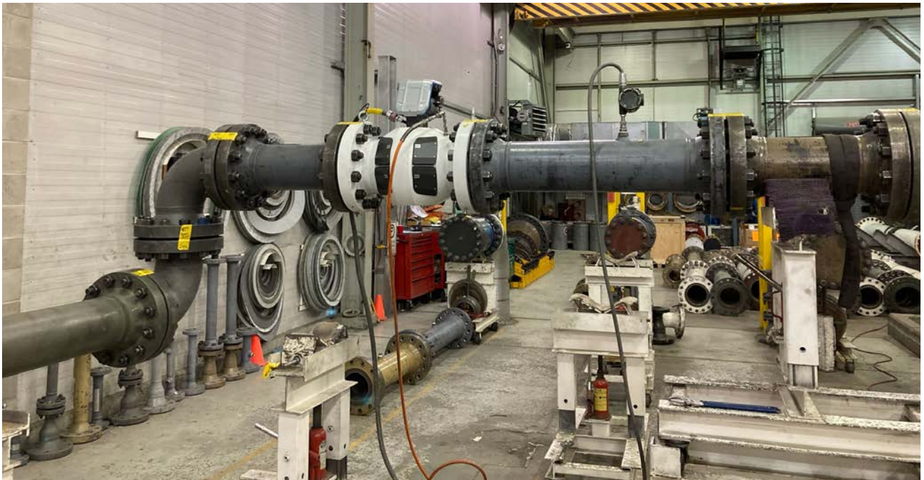
Fig. 25: FLOW SIC600-XT Forte - "double elbow out of plane right" testing with 3D w/o FC
