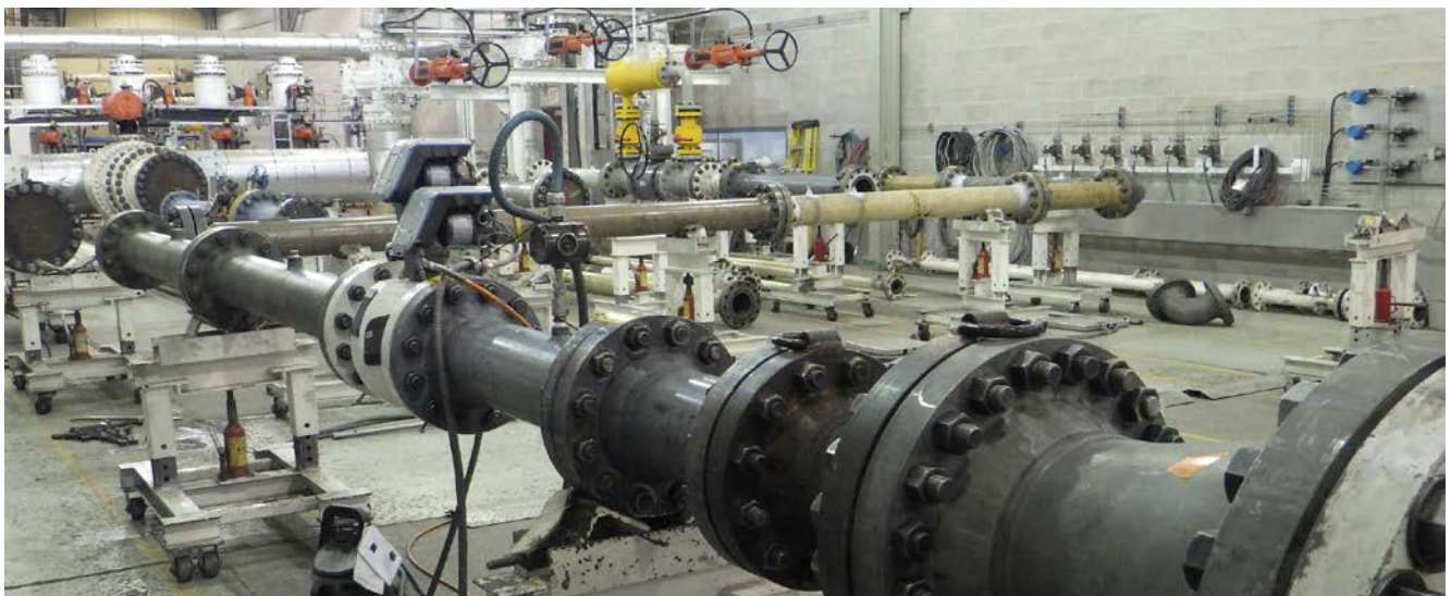
Fig. 15: FLOWSIC600-XT 2plex - “single elbow left” testing with 10D|CPA50E|10D
