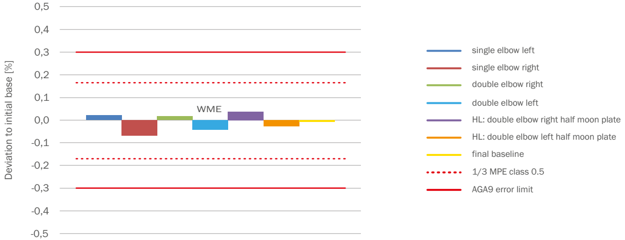
Fig. 27: WME of FLOWSIC600-XT Forte, 8 inch, 8-path; 5D inlet w/o flow conditioner, 14.5 psi
