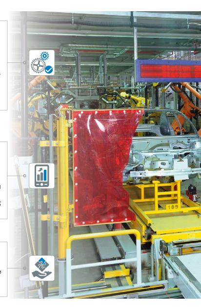
Safe Portal Solutions from SICK ensure flexible, efficient safeguarding for automated material transfer stations. Operating with up to eight simultaneous protective fields, vertically installed safety laser scanners detect people gaining unauthorized access of any kind.
