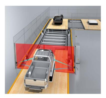
Safe Portal Solutions can be expanded, for instance, to allow passage of component baskets moving on skillet conveyors.
