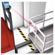
Identifying goods by means of bar codes The CLV650 bar code reader with autofocus adjustment reads the bar code on the grid box and supplies the data to a central computer, which assigns the AGV the new storage space and thus the drive path.
