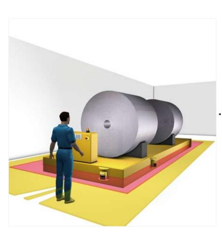
Non-contact comprehensive protection Four S3000 safety laser scanners provide the automated heavy load vehicle with allaround protection for humans and against collisions with materials in its path. Protective and warning fields do not need to be changed according to the speed because the AGV only moves very slowly.
