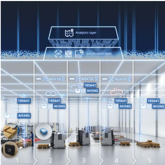
Fig. 9: Indirect localization of high volume, small assets involves linking the identification data of those assets with the location data of larger movable objects, for example manned forklift trucks.
