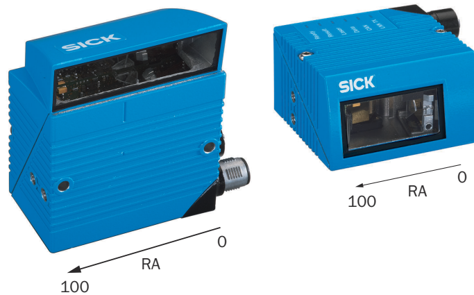
Figure 22: Counting direction of the reading angle RA in the scan plane: For devices in the IP65 standard housing with side viewing window (left) and front viewing window (right)
