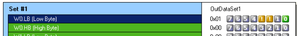
Figure 46: Network output bits without assigned tag name in the online process image
