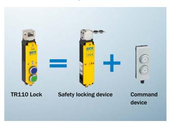
A further variant of the TR110 Lock is characterized by its integrated display and control elements. Illuminable pushbuttons or indicator lights in the switch cover make it possible to trigger control signals such as door requests or acknowledgments, directly on the safety switch. There is no need for an additional command device.
