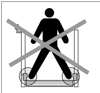
Fig. 14: Opposing sensors must not be capable of simultaneous activation
