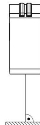
*Sensor should view perpendicular to the foil (90°). Background is faint black or empty at least 1m distance. Scanning range (front of sensor to foil) 90...120mm.*
