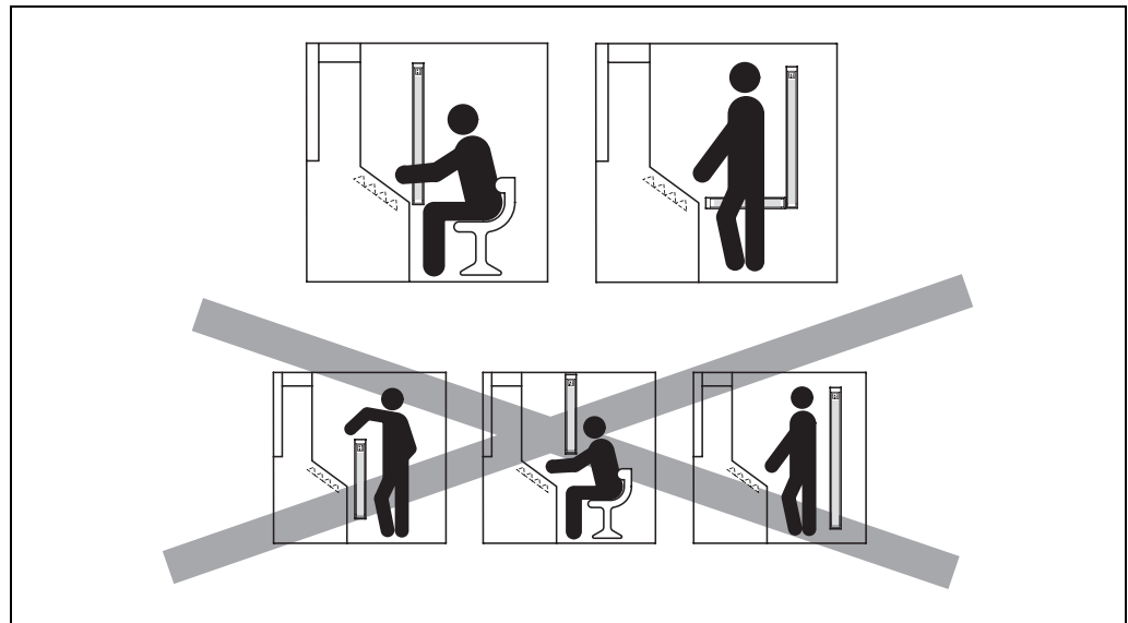
Fig. 2: The mounting position must prevent the following: reaching over, under, around and stepping behind
