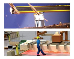
Falling chips do not trip the safety light curtain.
