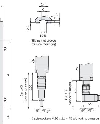
Dimensional drawing C4000 without extension connection, sender (receiver, mirror image)
