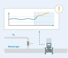
If the gas composition changes due to the incorporation of other gas types, e.g. hydrogen, the operator receives a status notification as soon as the GQI exceeds the configured permissible deviation. Any changes in gas quality can thereby be detected.
