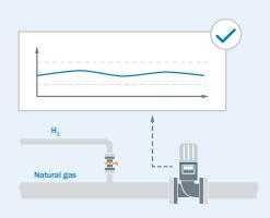
While commissioning the FLOWSIC500, the current gas composition and a permissible deviation can be configured via the Gas Quality Indicator (GQI) in FLOWgate<sup>TM</sup>. The gas quality is constantly monitored.
