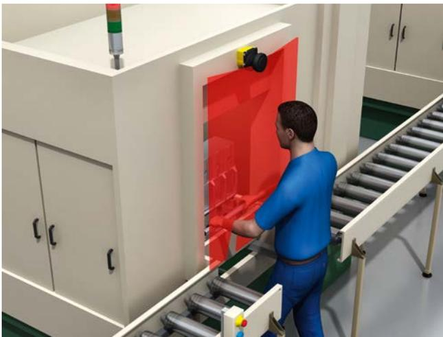
Hazardous point protection: If a person reaches into the hazardous area, the microScan3 will recognize this by detecting their arm.
