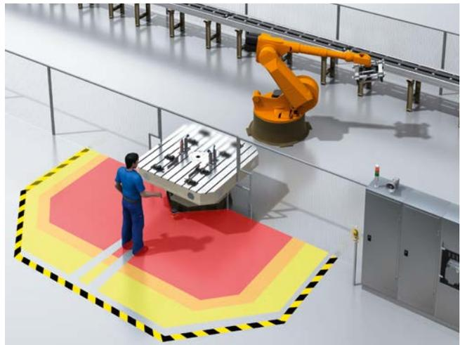
Stationary hazardous area protection: The microScan3 can tell if a person is approaching or standing in the hazardous area by detecting their leg.
