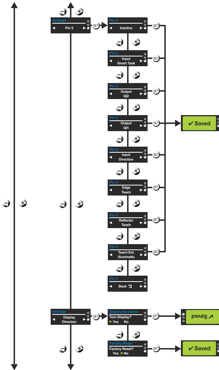
Figure 6: Menu tree with Settings / Pin 5 / Display Direction menu
