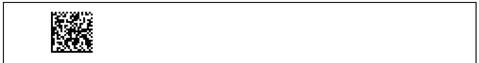
Fig. 6-18: 2D code sample: Data Matrix ECC200; cell size 0.3 mm (11.8 mil)
