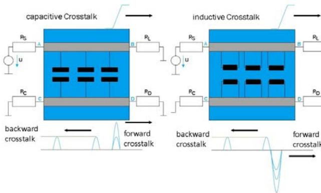
Fig. 1 – Cable model for capacitive and inductive crosstalk and signal propagation (forward and backward) [1]
