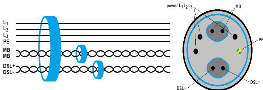
Fig. 2 - general configuration of a motor cable and principle location of the pins within a connector; a separate DSL-shield-connection is required for coupling connectors within the line
