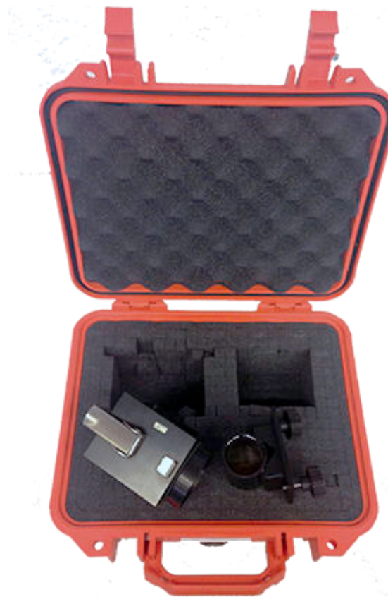
Figure 8: CO test cell with holder in transport case
