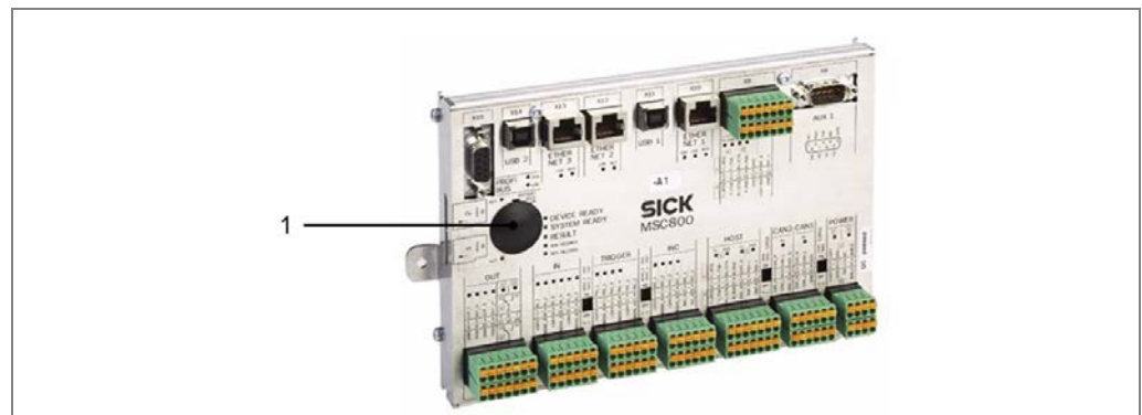
Fig. 93: Position of the battery in the MSC800 controller
