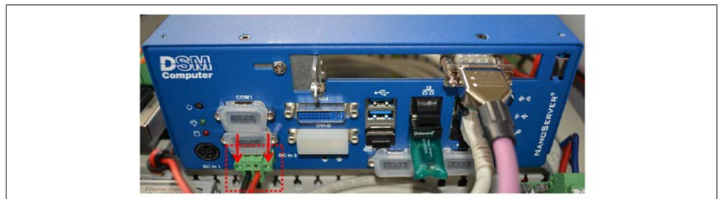
Fig. 96: Removing the VMC800: Unplugging the supply connection
