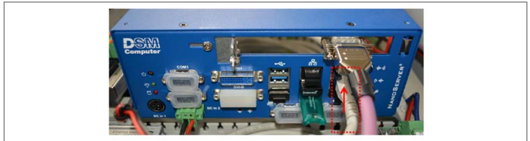
Fig. 97: Removing the VMC800: Unplugging the Ethernet cable
