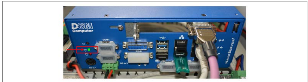
Fig. 77: Checking the operational readiness of the VMC800
