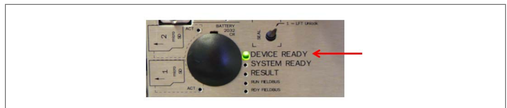
Fig. 76: Checking the operational readiness of the MSC800
