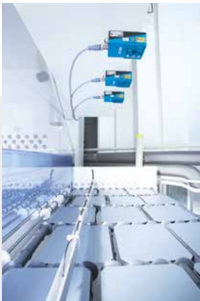
2D vision solutions from SICK monitor position and possible breaks when handling solar cells.
