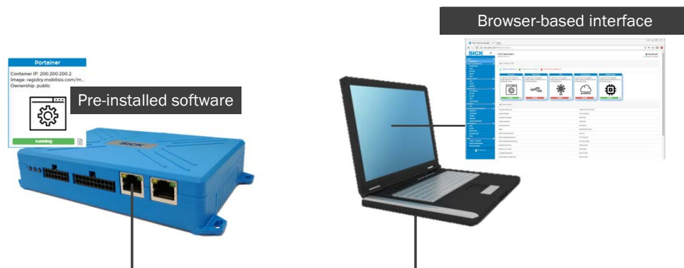
Fig. 29: Connecting the TDC-E terminal device to the browser
