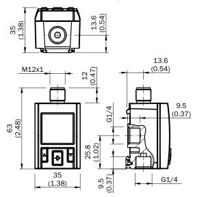
Bottom side: push-in fitting for 4 mm pneumatic hose, back side: thread G 1/4 female
