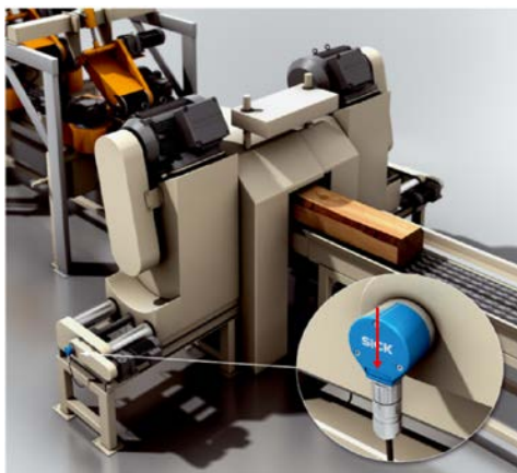
Fig. 7: Advantageous arrangement of the connection. Cable runs or shocks in the direction of the arrow do not cause the encoder to rotate
