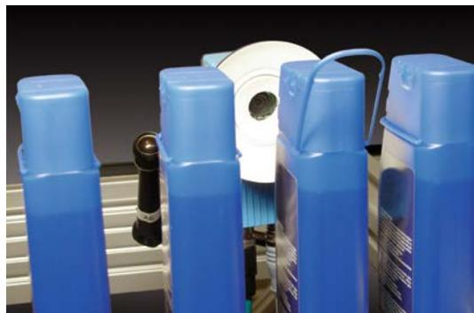
Bottle inspection: molded details and alignment verification
