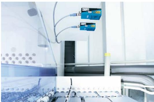
Solar wafer edge damage detection
