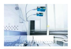
Solar wafer edge damage detection
