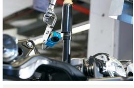
Verification of hole presence as well as nuts, safety springs and washers
