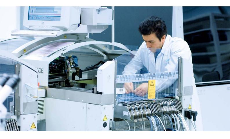
The Inspector PIM-series provides high-speed positioning, inspection and measurement. Its multi-functional vision toolbox solves a wide range of quality control applications and improves production efficiency. The PIM-series combines smart camera functionality with the ease of use of a vision sensor.
