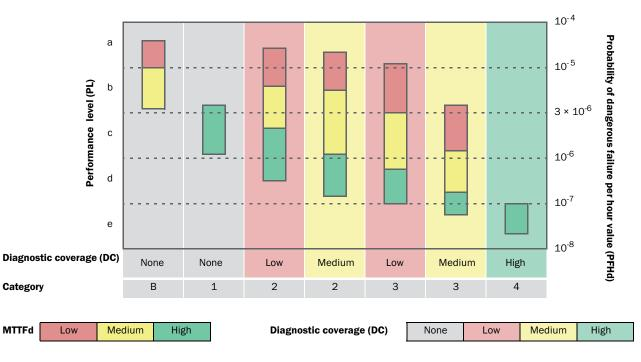
A performance level of d can be achieved with a dual-channel control system (category 3), for example. This can be reached either with components of good quality (MTTFd = medium) if almost all faults are detected (DC = medium) or with components of very good quality (MTTFd = high) if many faults are detected (DC = low).
