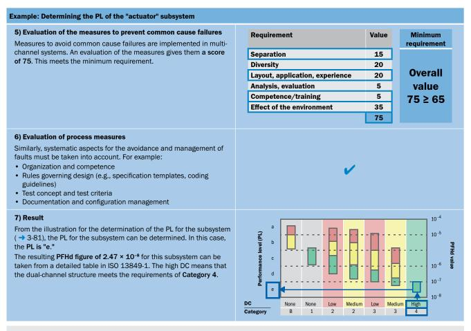
→ With the resulting data for the subsystem, it is now possible to determine the performance level of the entire safety function achieved (see "Determining the performance level (PL) achieved as per ISO 13849-1" → 3-81).
