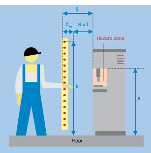
Parameters for determining the required minimum distance for reaching through
