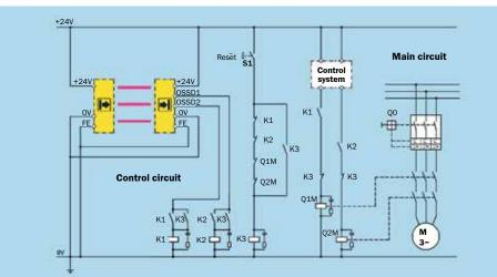
Using individual auxiliary contactors with positively guided contacts, it is possible to design control systems with any level of complexity. Redundancy and monitoring by positively guided contacts are features of this safety principle. Wiring provides the logical operators.
