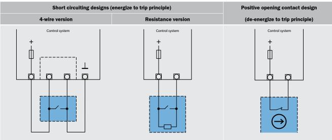
Here, the activation of the protective device triggers a short-circuit. In the case of the 4-wire version, a circuit is short-circuited (a few Ohms). In the case of the resistance version, a change from a set resistance (a few kOhms) is detected. These designs require more complex evaluation.
