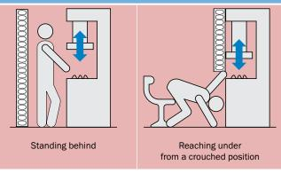
Once the minimum distance between the protective field and the nearest hazardous point has been calculated, the protective field height required must be determined in a further step. This ensures the hazardous point cannot be accessed by reaching over the protective field before the hazardous machine function has ceased.
