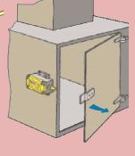
Flawed: The position switch will not always open the safety circuit, e.g., if the plunger is sticking due to encrusted deposits or lubricating oil residue that has solidified.
