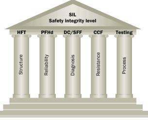
The safety integrity level achieved for a subsystem is made up of the following parameters:
