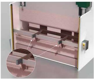
Fixed blanking of light curtain beams on a trimming press.
