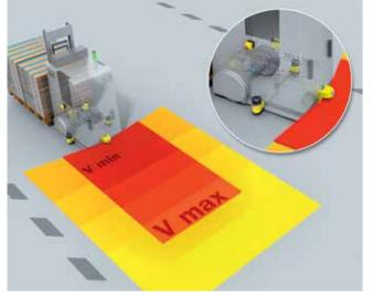
Speed monitoring for protective field switching on an automated guided vehicle
