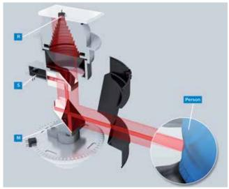
Basic structure of a laser scanner
