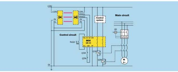
Safety relays combine one or more safety functions in one housing. They generally have automatic monitoring functions. They can also have signaling contacts.
