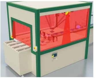
Camera-based protective device
