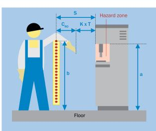
Parameters for determining the required minimum distance with possibility of reaching over
