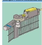
**Safe:** The opening of the protective door positively actuates the mechanical plunger of the position switch. This opens the safety circuit.
