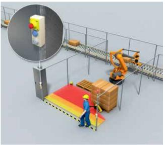
The position of the reset pushbutton allows a full view of the hazard zone for the resetting of the protective device.
