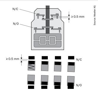
Contact system of a contactor with positively guided contacts. A normally open contact is welded.
