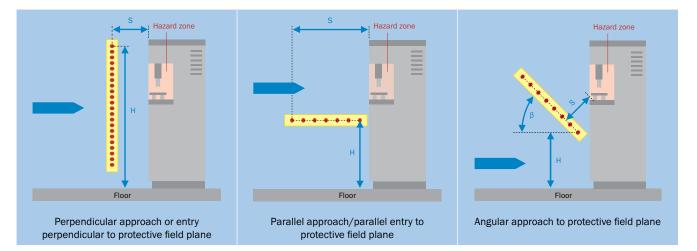
After the ESPE has been selected for the safety function "initiating a stop," the required minimum distance between the ESPE's protective field and the nearest hazardous point is to be calculated.
