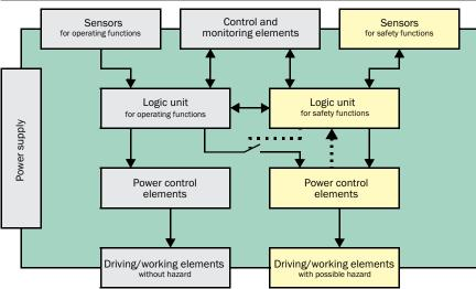
The safety-related parts of control systems are to be selected to suit the safety functions and the necessary level of safety. These parts include sensors, logic units, power control elements, for example, as well as drive and work elements. This selection is generally made in the form of a safety concept.
