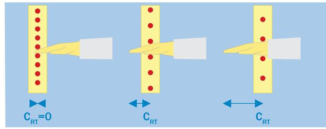
The figure shows an example of depth penetration factor before detection at safety light curtains with different detection capabilities.
