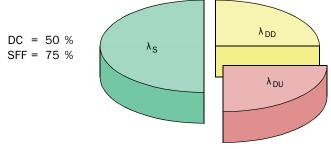
The "safe failure fraction" (SFF) consists of the diagnostic coverage DC  $(\lambda_{_{DD}}/\lambda_{_{DU}})$  and the "safe failure" fraction  $(\lambda_{_S})$ .
