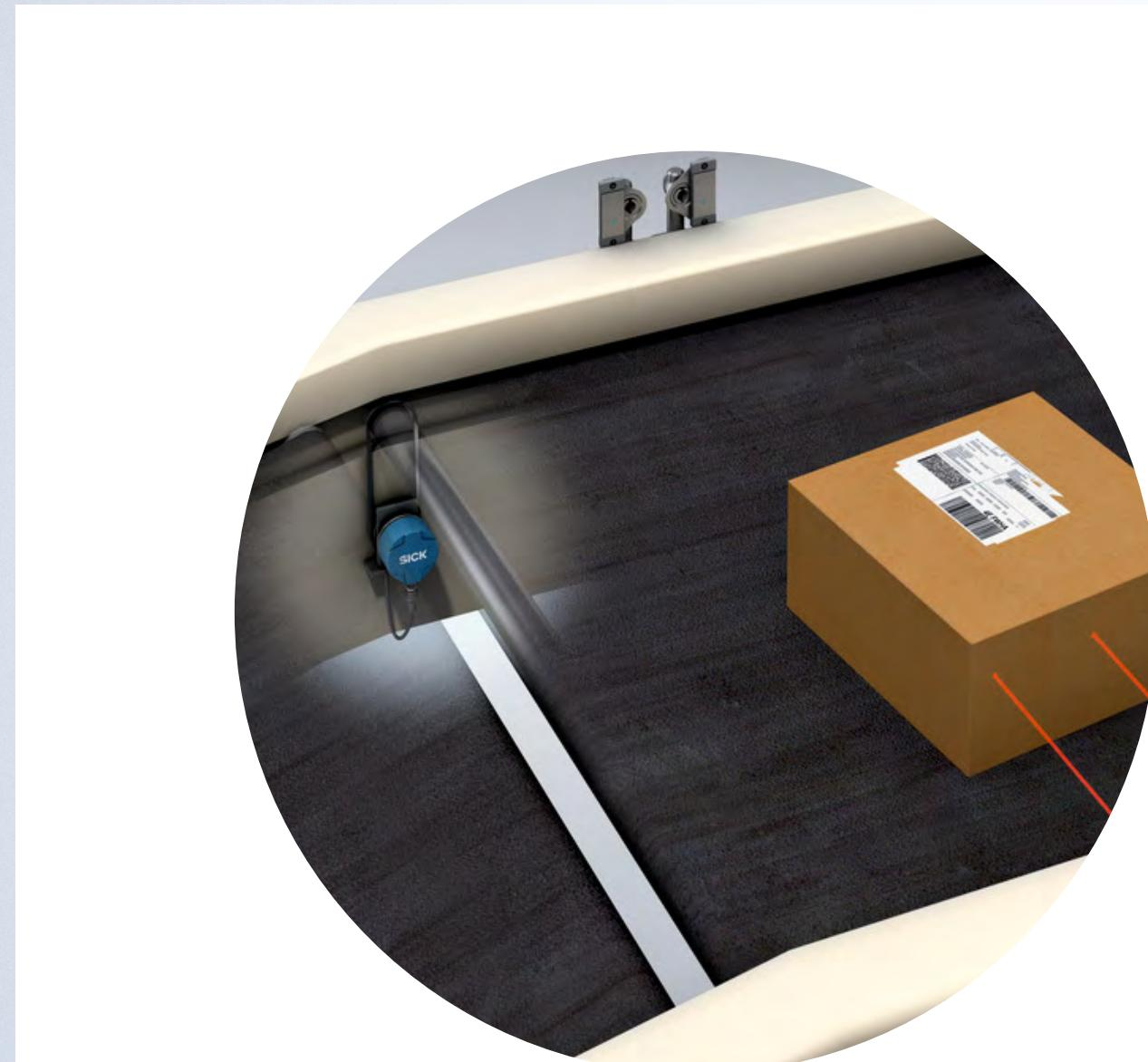
② Positioning when feeding to the palletizer robot
