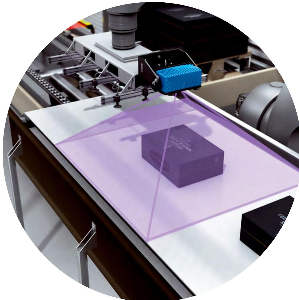
**Contour measurement for pallet loading**
