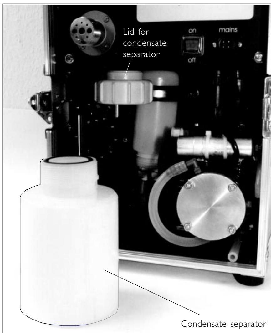
Fig. 6201 Removed Condensate separator
