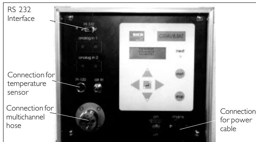
Fig. 3502 Connections to the evaluation unit
