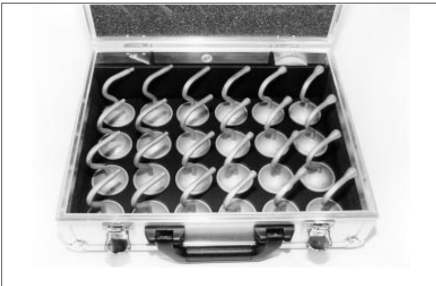
Fig. 2408 Specially designed case with a set of LC dust collectors
