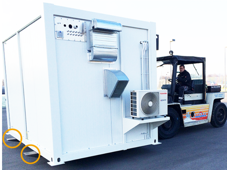
Fig. 9: Fork tips protrude over the edge
