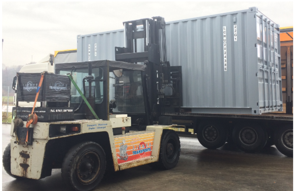
Fig. 27: Sea container unloading
