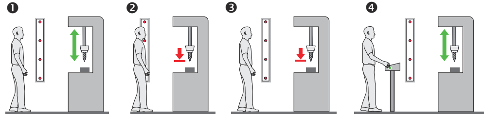
Figure 13: Schematic representation of operation with restart interlock
