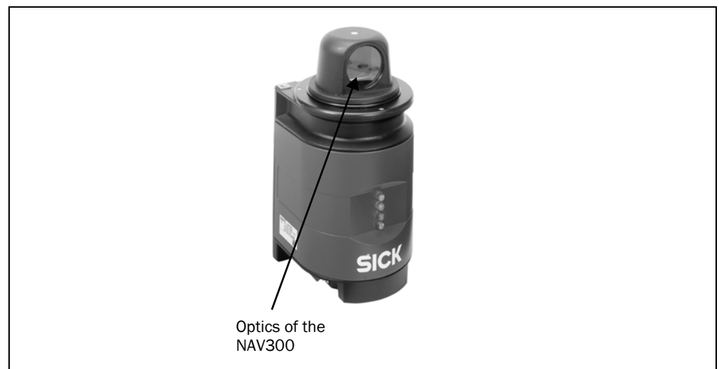
Fig. 25: Optics for the NAV300
