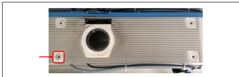
Fig. 33: Mounting the camera system: inserting the screw into the fitting
