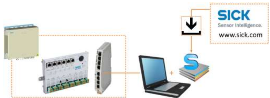
Fig. 74: Establishing the configuration PC – SIM2000-2 Prime system controller connection
