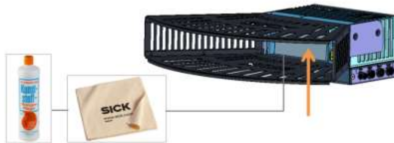
Fig. 76: Cleaning the front screen of the 2D LiDAR sensor
