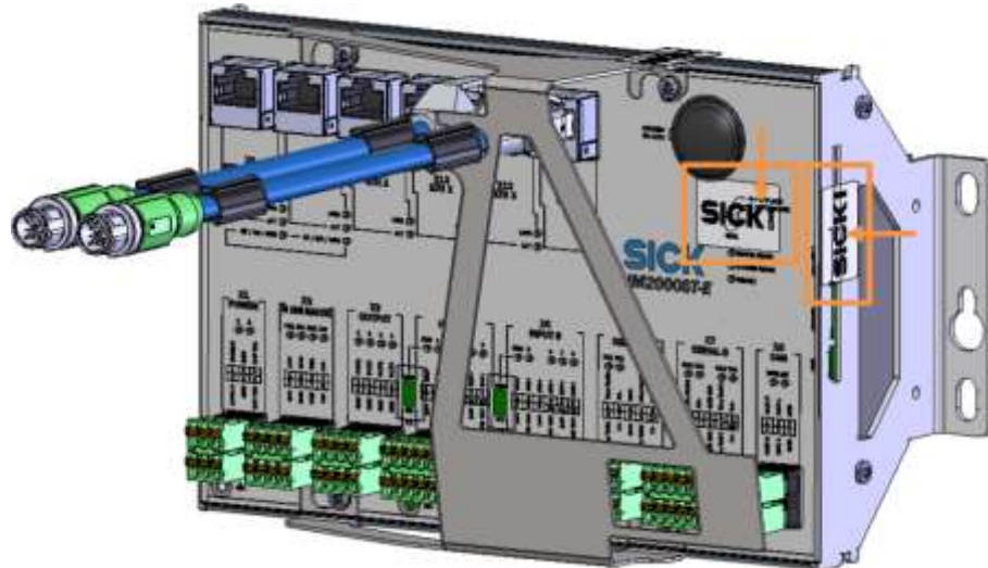
Fig. 39: Securing the alibi memory card with security seal on the card slot of the SIM2000-2 Prime controllers and securing the calibration switch with security seal on the switch on the front of the housing
