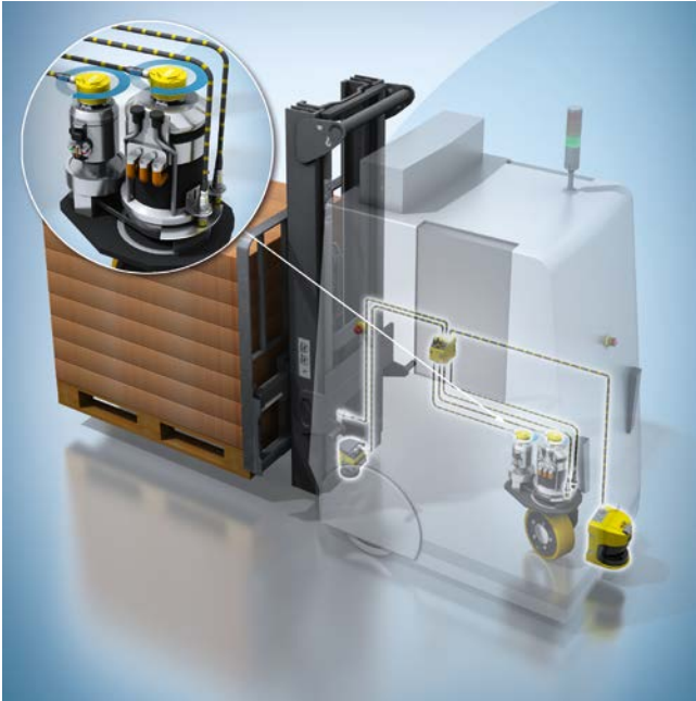
Detection of rotative movements on an automated guided vehicle.
