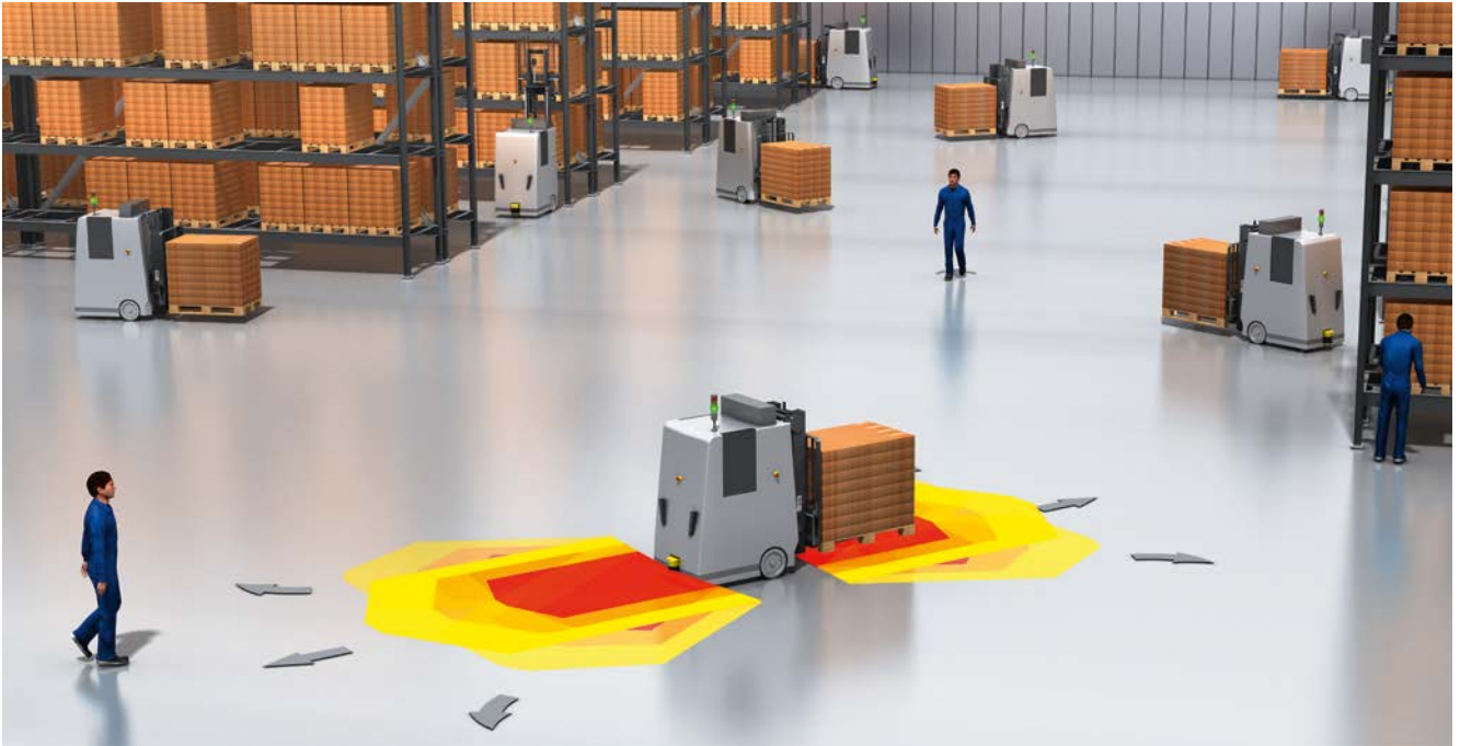
Automated guided vehicles – protective field switching via steering angle detection.
