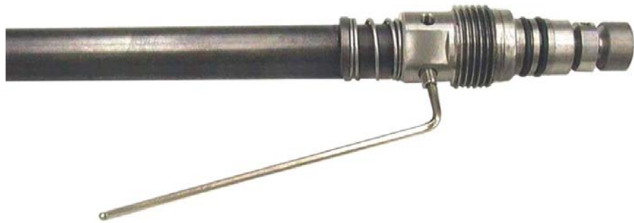
Fig. 3.13: Mounting the transducer assembly (1) to the docking rod (3)
