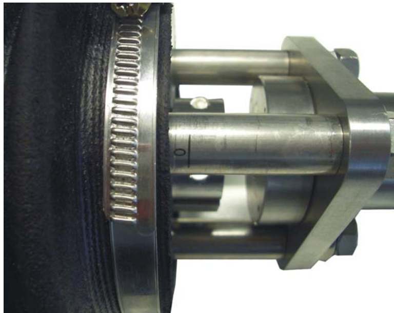
Fig. 3.18: Bellows flange on the pressure side (5.7)
