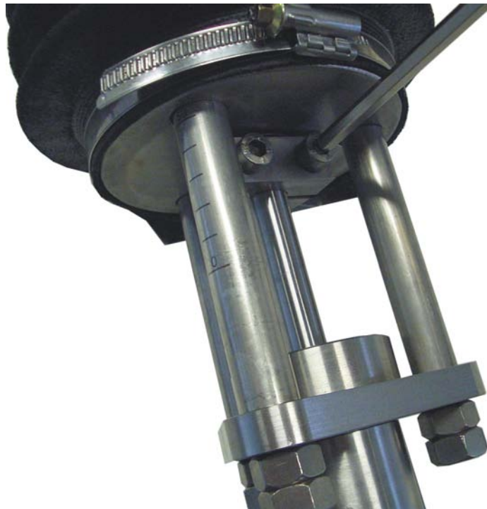
Fig. 3.12: Undoing the coupling (5.4) to dismount the docking rod (3)
