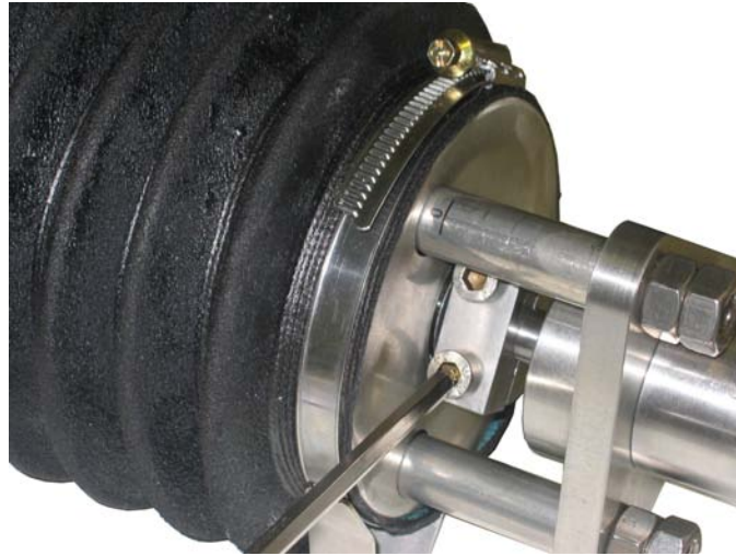
Fig. 3.8: Connecting the spindle assembly (5) and docking rod (3)
