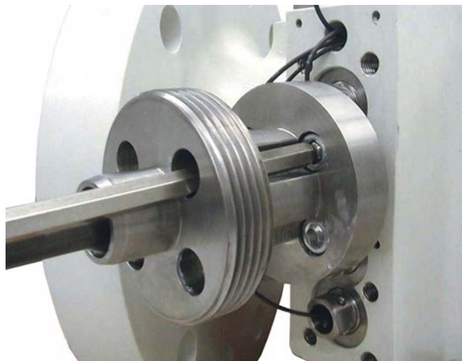
Fig. 3.4: Mounting the adapter (2) to the meter body
