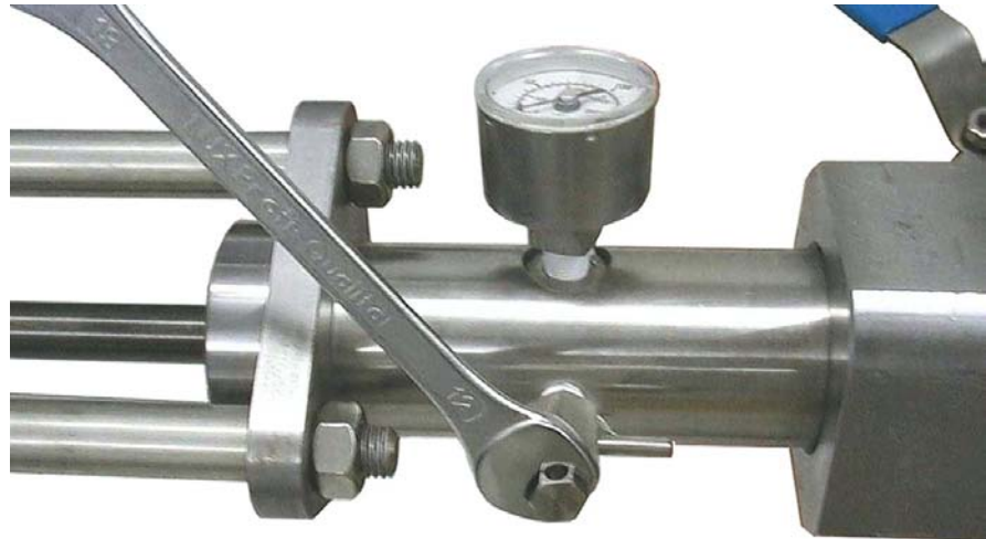
Fig. 3.19: Opening the bleed valve (5.3)
