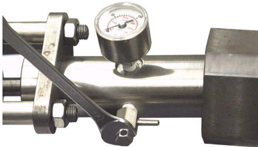
Fig. 3.10: Opening the bleed valve (5.3)
