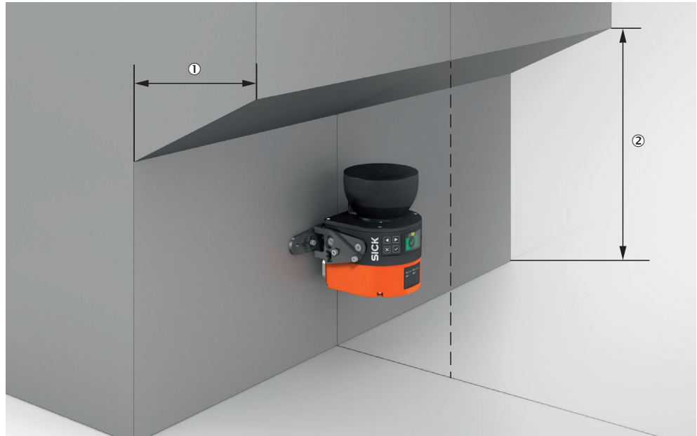
Figure 19: Mounting in an undercut (example)
