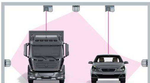
Axle counting using 2D LiDAR sensors mounted on the side of the road.
