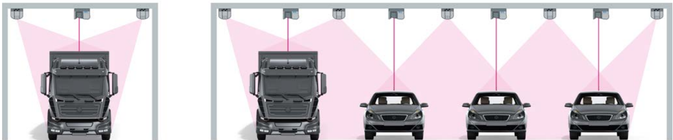
Depending on the number of lanes, the system is individually adapted.
