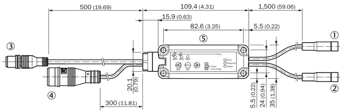
Figure 34: Dimensional drawing – FlexChain Host Standard
