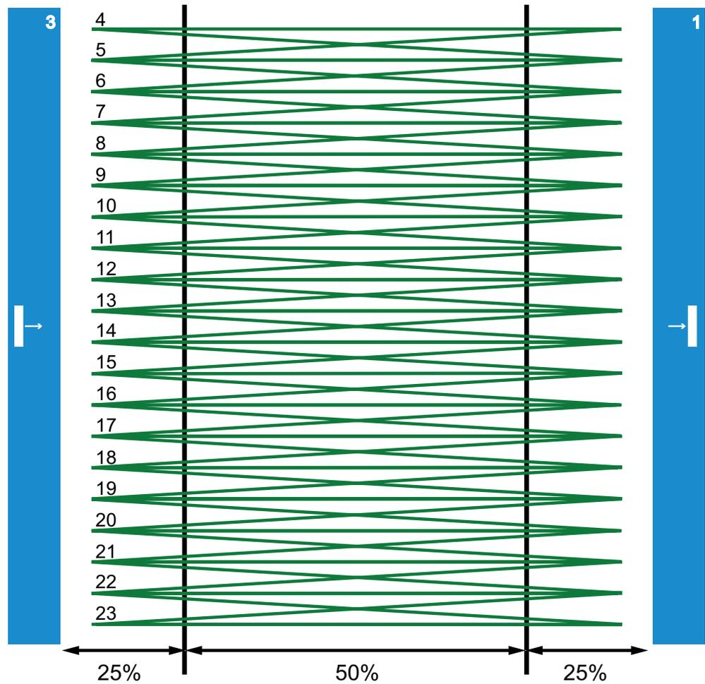
Figure 14: Cross beam, to improve the resolution in the middle 50%
