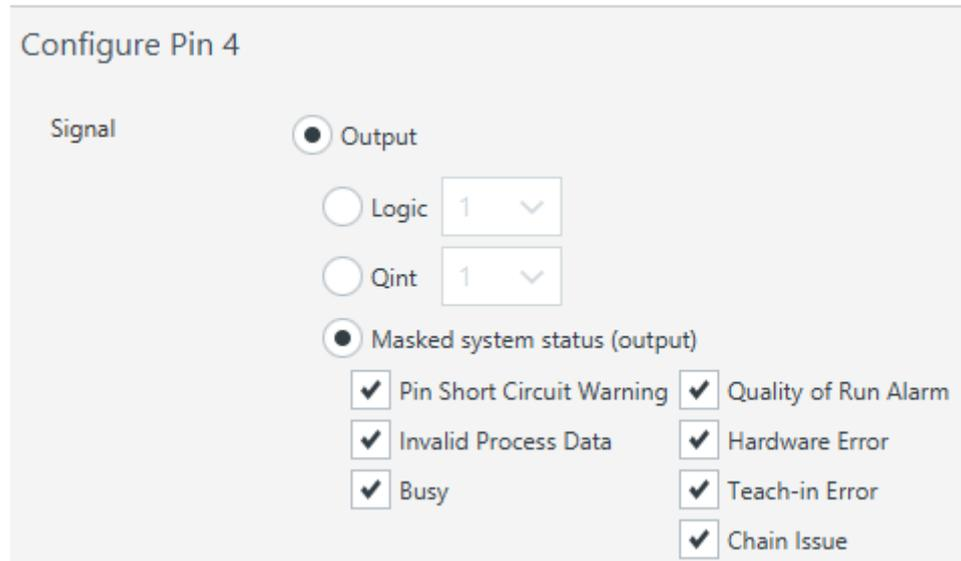
Figure 31: Configuration of PIN 4 / Masked System Status
