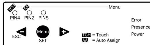
Figure 41: FlexChain Host IO-Link Standard control panel
