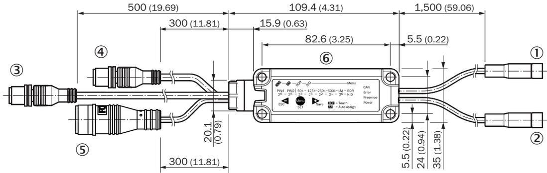
Figure 35: Dimensional drawing - FlexChain Host CANopen
