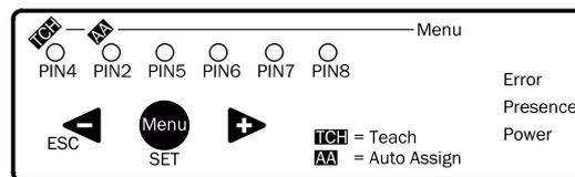
Figure 42: FlexChain Host IO-Link Advanced control panel
