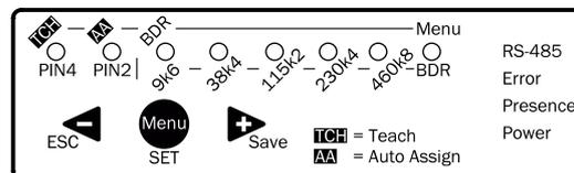
Figure 43: FlexChain Host RS485 control panel
